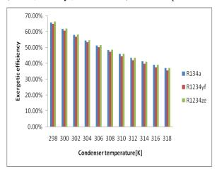
Fig: 8. Variation of exergetic efficiency with condenser temperature Conclusion
