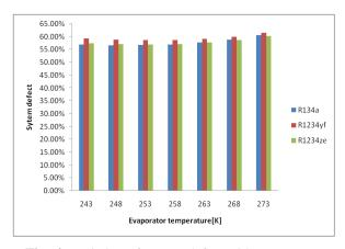
**Fig: 4.** Variation of system defect with evaporator temperatures
