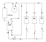
Fig: 1 (a). Schematic diagram of actual multievaporator with single compressor and single expansion valve and LVHE
